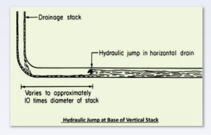
To alleviate the backflow at the lower part of the downpipe, the following measures are suggested:
